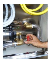
Empty all water from the tank in order to eliminate the soot accumulated in the unit. The operation must be performed before starting the fire in the oven with switched off machine.
