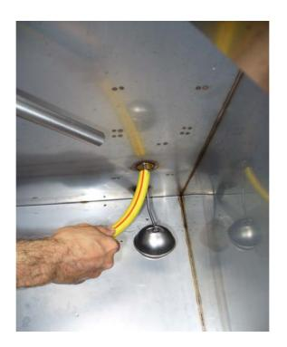
direct the jet of water on the water level switched placed on the left in the lower part of the tank, carefully clean hole and arm of the water level switch and check that it moves up and down correctly.
