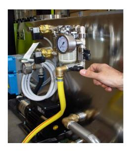
Open the auxiliary tap connected to the hose
