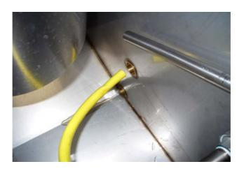
the two holes in the low part of the unit are the water drain gate (lower hole) and water expulsion at level to sewer (upper hole)
