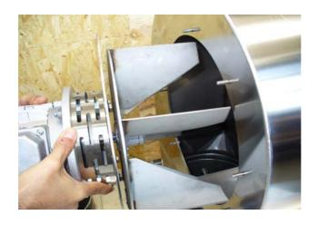
reposition the fan into the stainless steel spiral
