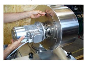
Unscrew the butterfly bolts to remove the motor coupled to the fan from the stainless steel spiral
