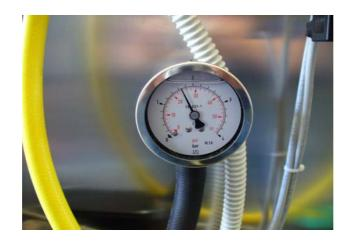
If the unit is working properly, the manometer above the pump shows a pressure around 2,0 bar
