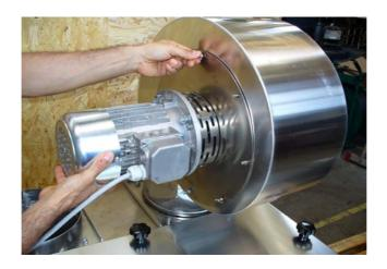
screw the butterfly bolts in order to block the fan on the stainless steel spiral.
