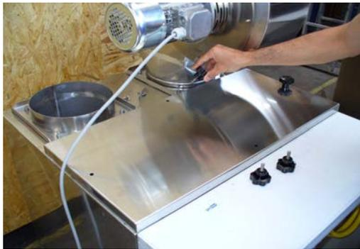
**Close the inspection window by means of the 4 fastening knobs**
