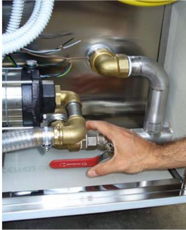
***Once the lever has been turned water level will start to lower until the tank is empty***
