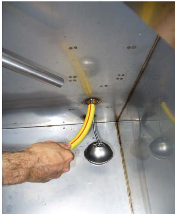
**direct the jet of water on the water level switch placed on the left in the lower part of the tank, carefully clean hole and arm of the water level switch and check that it moves up and down correctly.**
