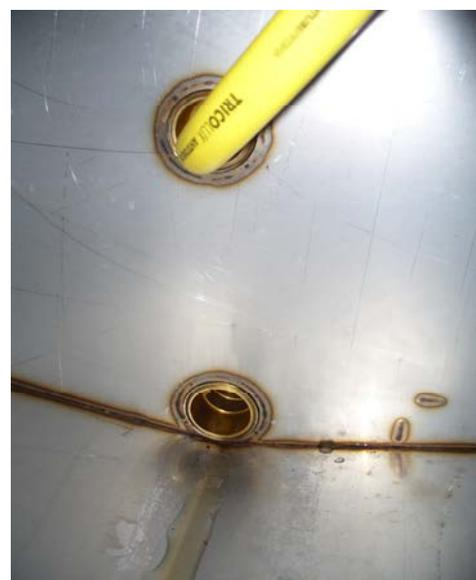
***The water expulsion hole must be always clean and free of muddy waste, so put the hose inside and clean with a high pressure jet of water.***
