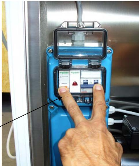
***The unit must be switched off at the end of the working time when the fire in the oven is extinguished***
