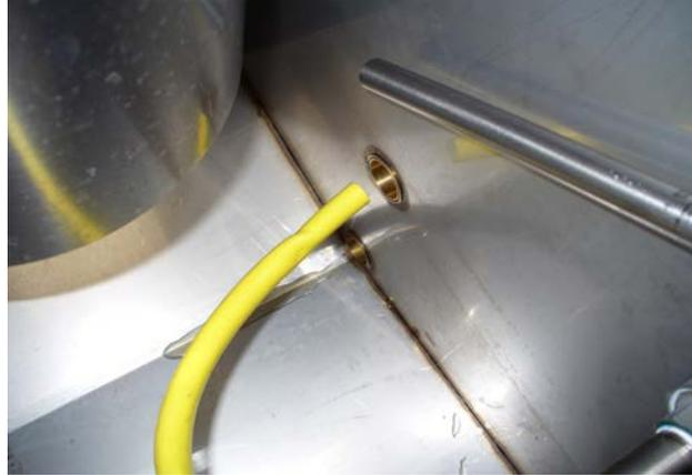
***the two holes in the low part of the unit are the water drain gate (lower hole) and water expulsion at level to sewer (upper hole)***
