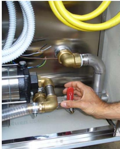
***When the tank is empty, turn the lever in the original position***
