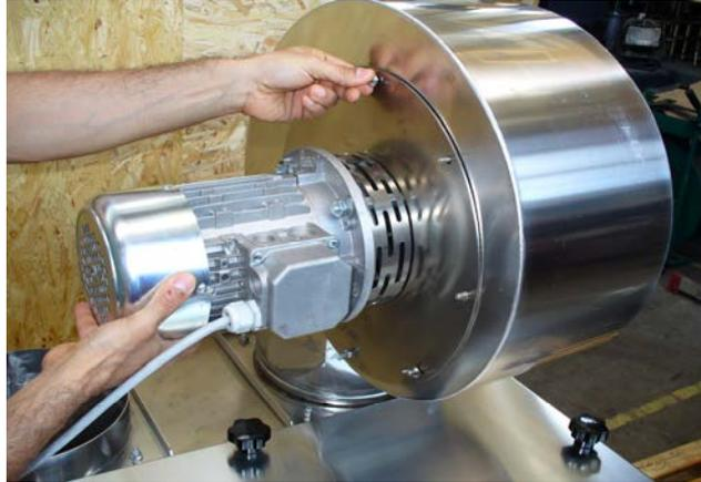
*Unscrew the butterfly bolts to remove the motor coupled to the fan from the stainless steel spiral*
